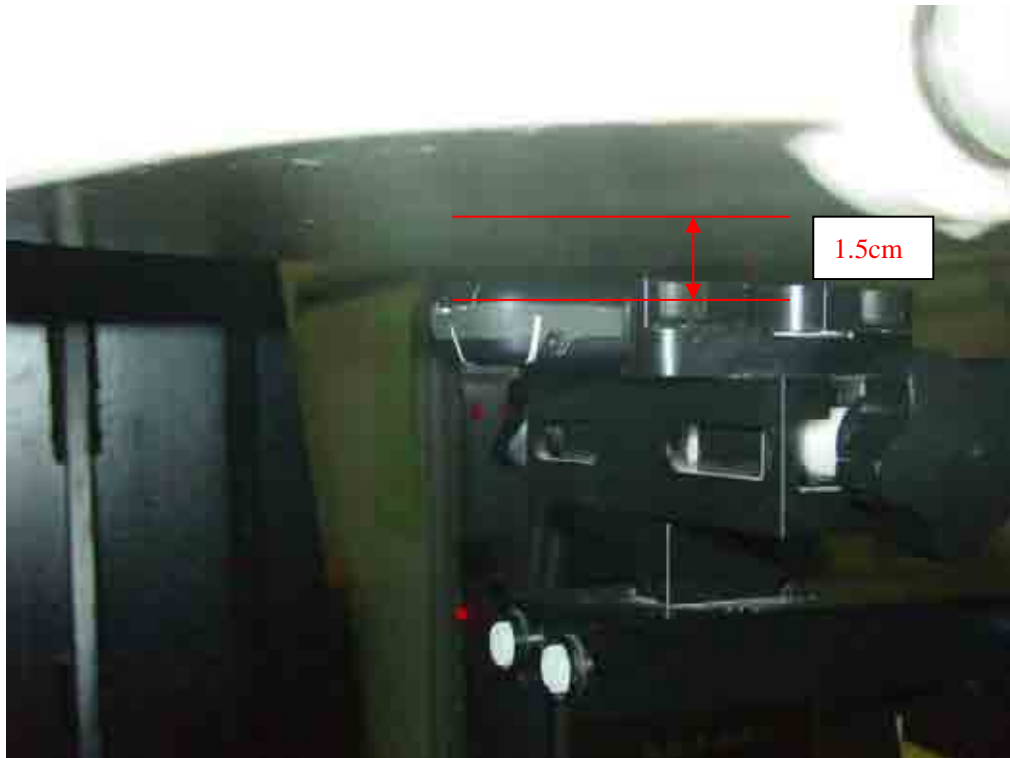
Picture B8: Body-worn Position (towards ground, the distance from handset to the bottom of the Phantom is
