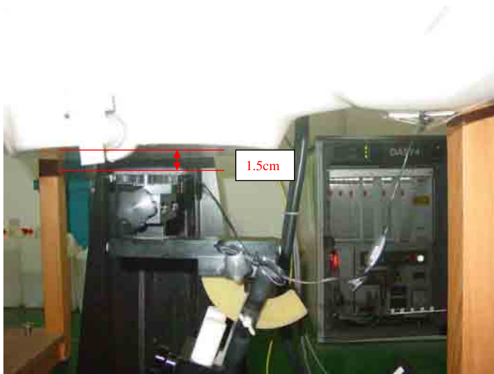
Picture B10: Body-worn Position with Headset (towards ground, the distance from handset to the bottom of the Phantom is 1.5cm)
