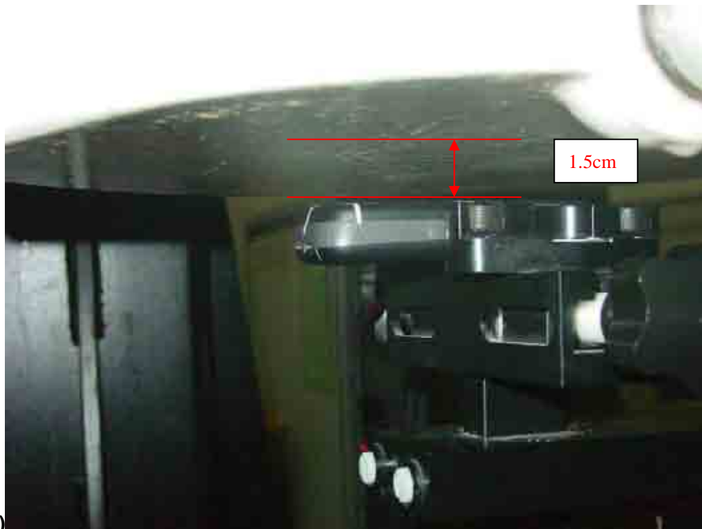
Picture B9: Body-worn Position (towards phantom, the distance from handset to the bottom of the Phantom is 1.5cm)
