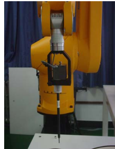
Picture4:ES3DV3 E-field probe
