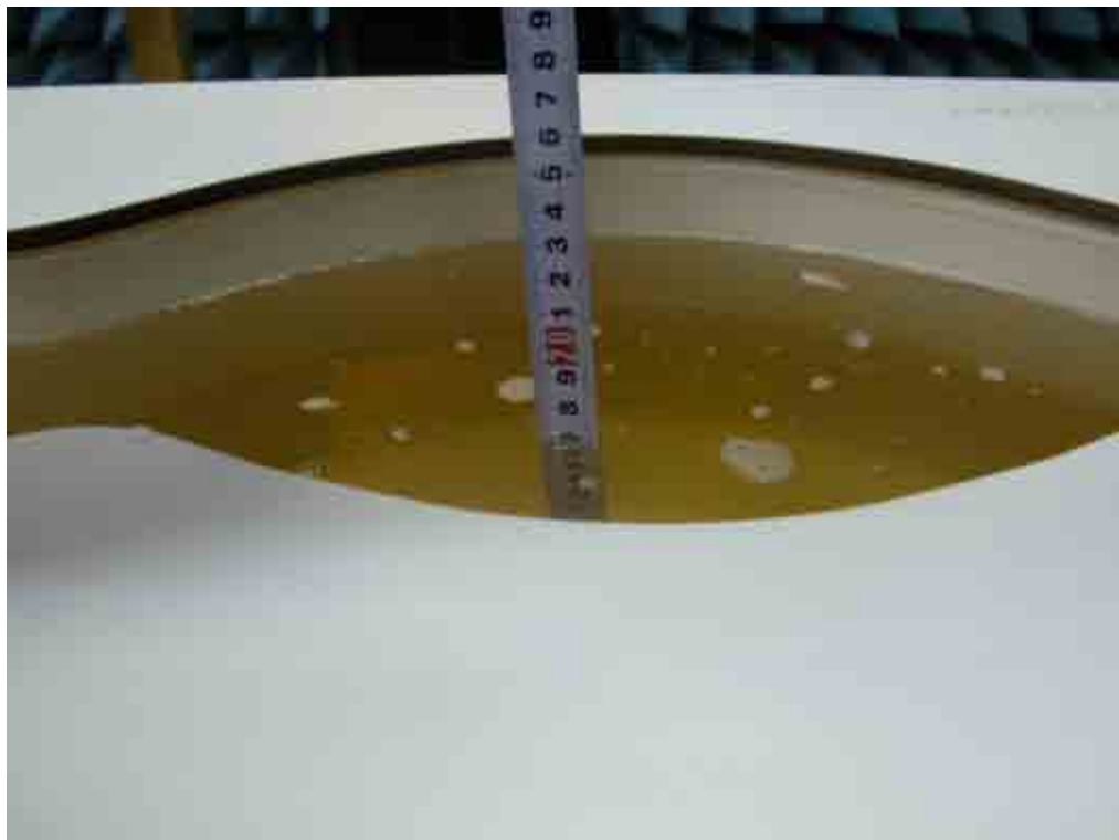
Picture B2: Liquid depth in the Flat Phantom (850 MHz)
