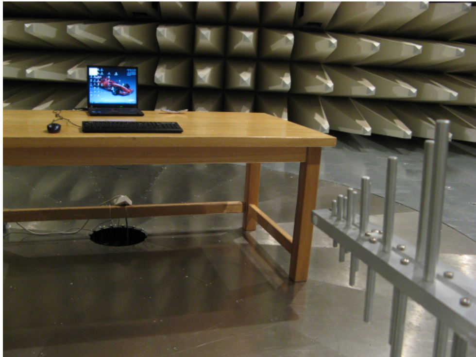
Pic C-3 Radiated Spurious Emission (USB Mode)
