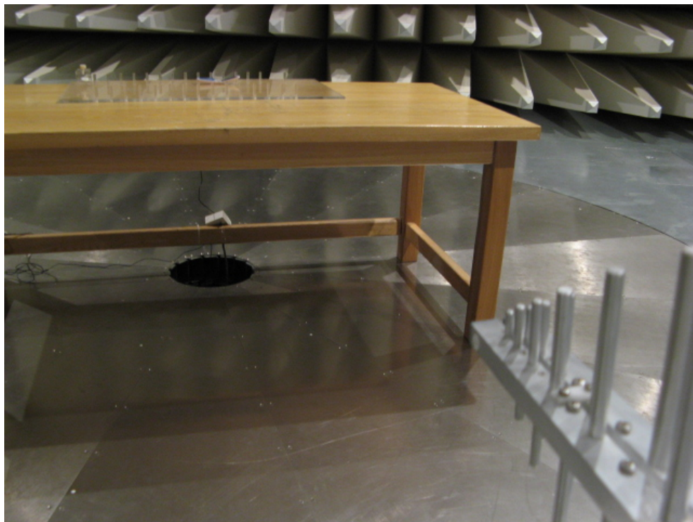
Pic C-2 Radiated Spurious Emission (Charging Mode)
