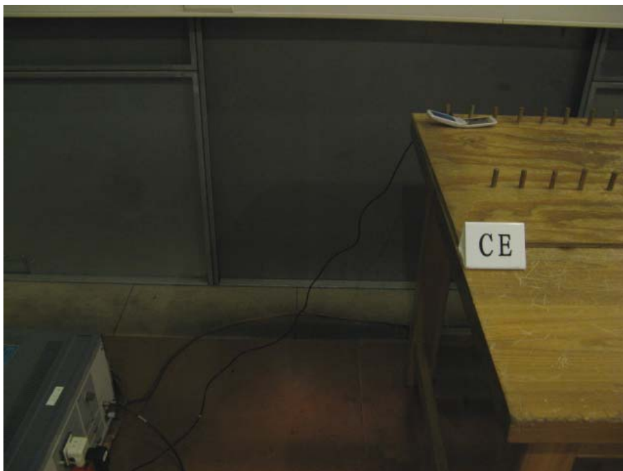
Photo of AC Powerline Conducted Emission Test
