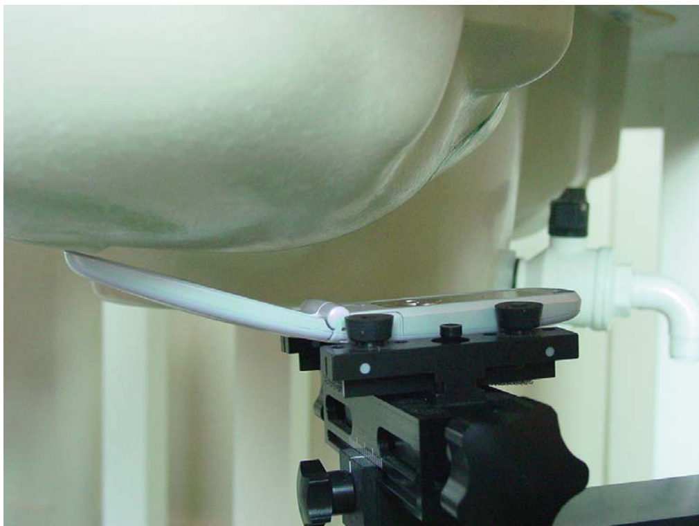
Picture B7: Right Hand Tilt 15° Position
