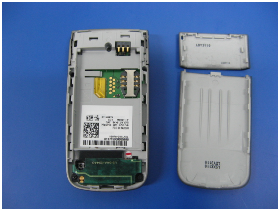
Mobile phone Disassembly
