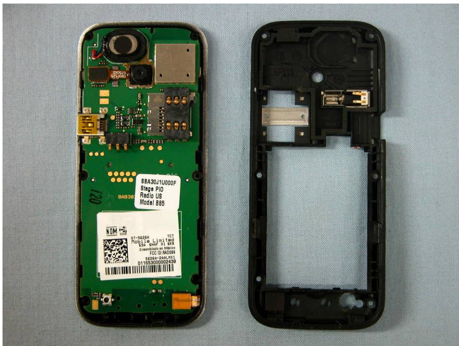
Mobile phone Disassembly
