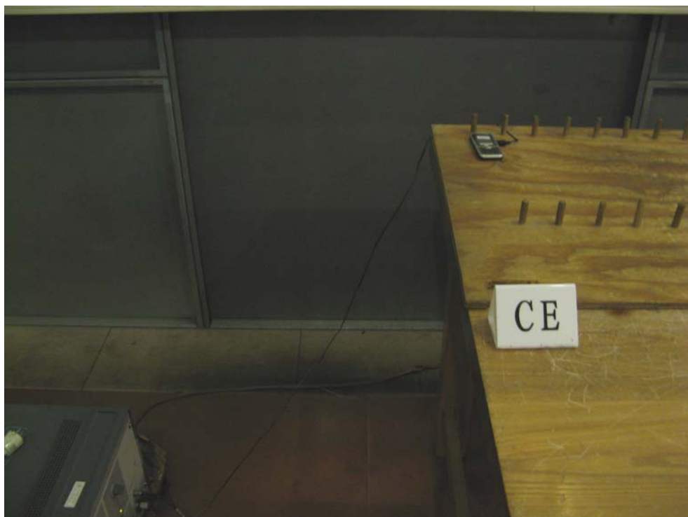
Pic C-2 Conducted Emission (with Charger)
