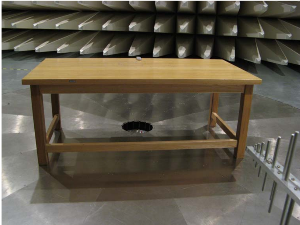
Pic 3 Radiated Spurious Emission for Part 15C
