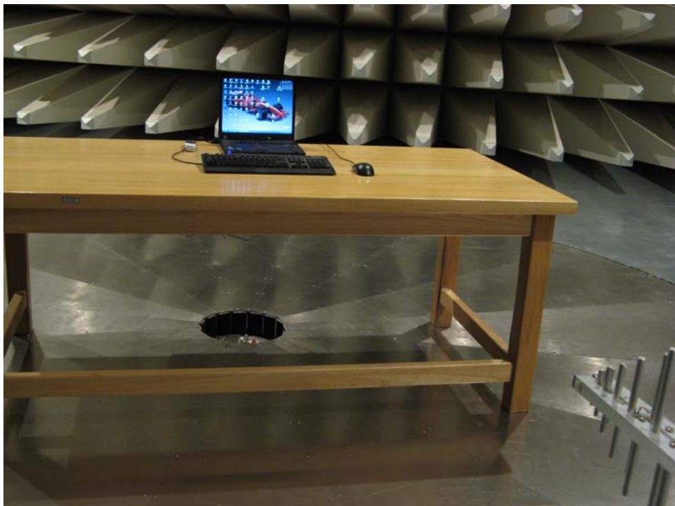
Pic 2 Radiated Spurious Emission for Part 15B
