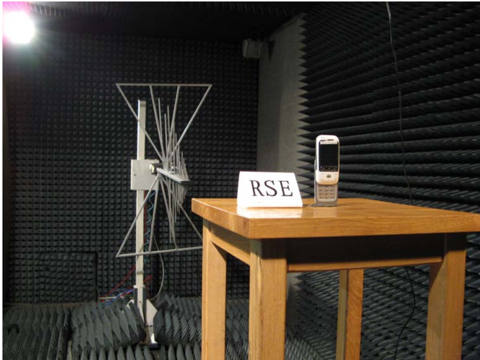
Pic 1 Radiated Spurious Emission for Part 22 24
