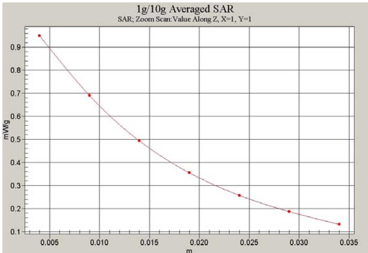
Fig. 74 Z-Scan at power reference point (850 MHz CH190)
