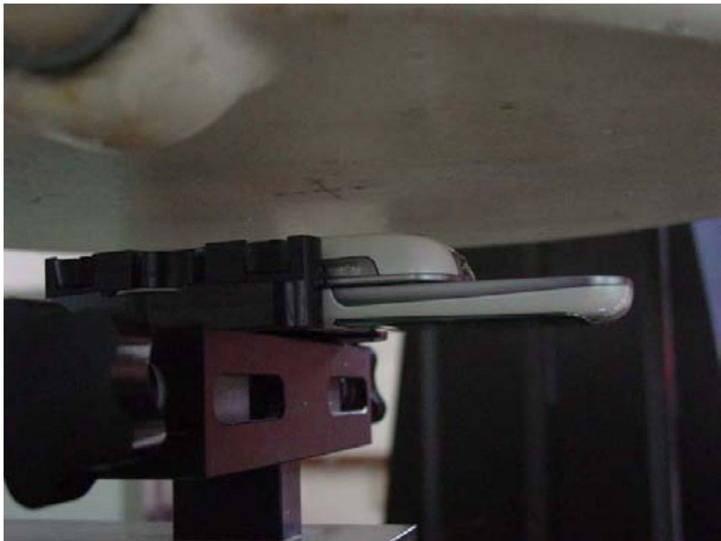
Picture B15: Body-worn Position with Slide up (towards ground, the distance from handset to the bottom of the Phantom is 1.5cm)
