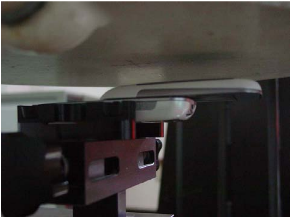
Picture B13: Body-worn Position with Slide up (towards phantom, the distance from handset to the bottom of the Phantom is 1.5cm)
