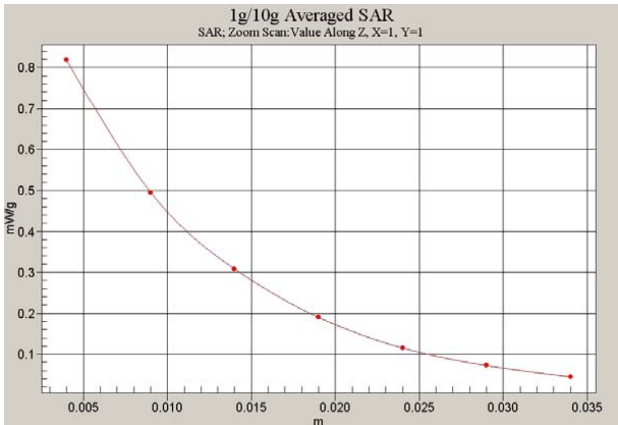
Fig. 14 Z-Scan at power reference point (850 MHz CH251)
