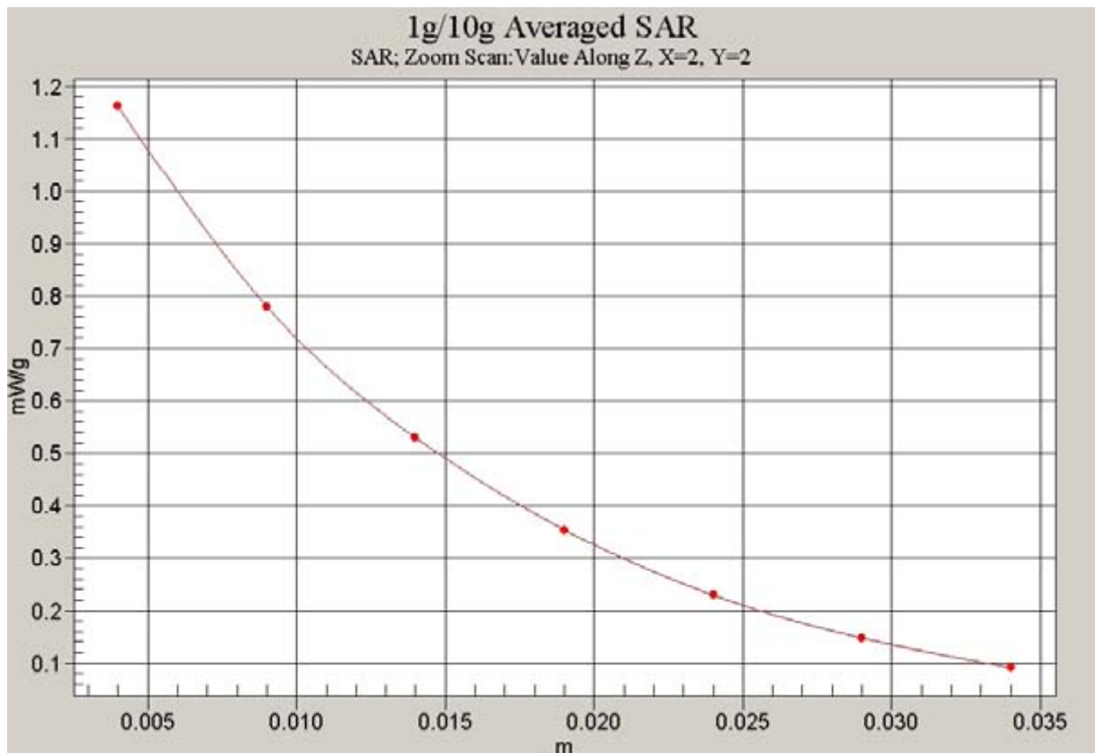
Fig. 18 Z-Scan at power reference point (850 MHz CH128)
