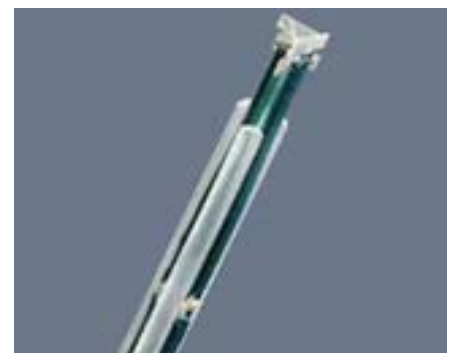
Picture 3: ES3DV3 E-field Probe
