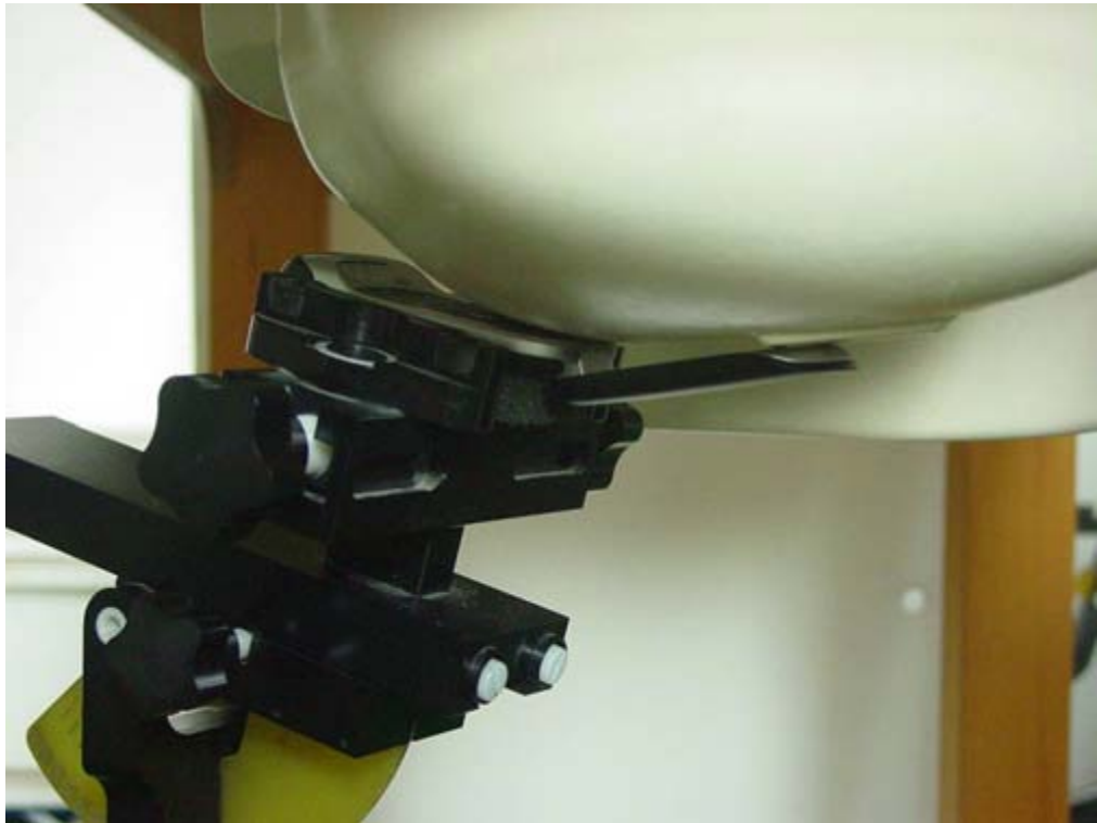
Picture B4: Left Hand Touch Cheek Position
