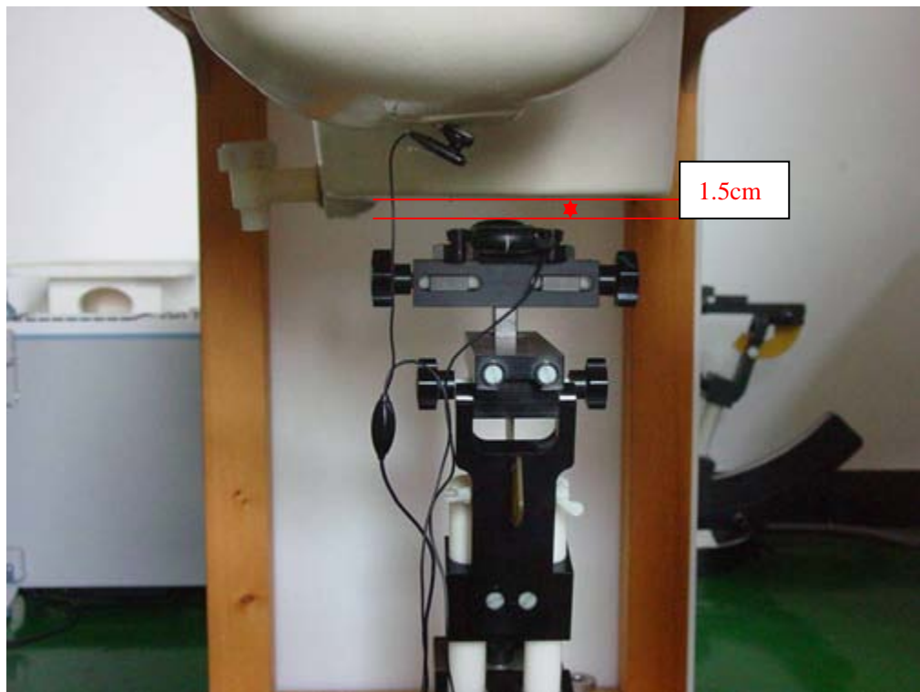
Picture B9: Body-worn Position with Headset (towards ground, the distance from handset to the bottom of the Phantom is 1.5cm)
