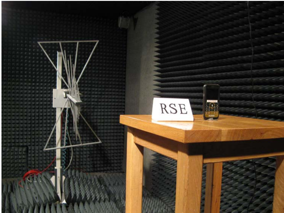
Pic 1 Radiated Spurious Emission Part 22 24
