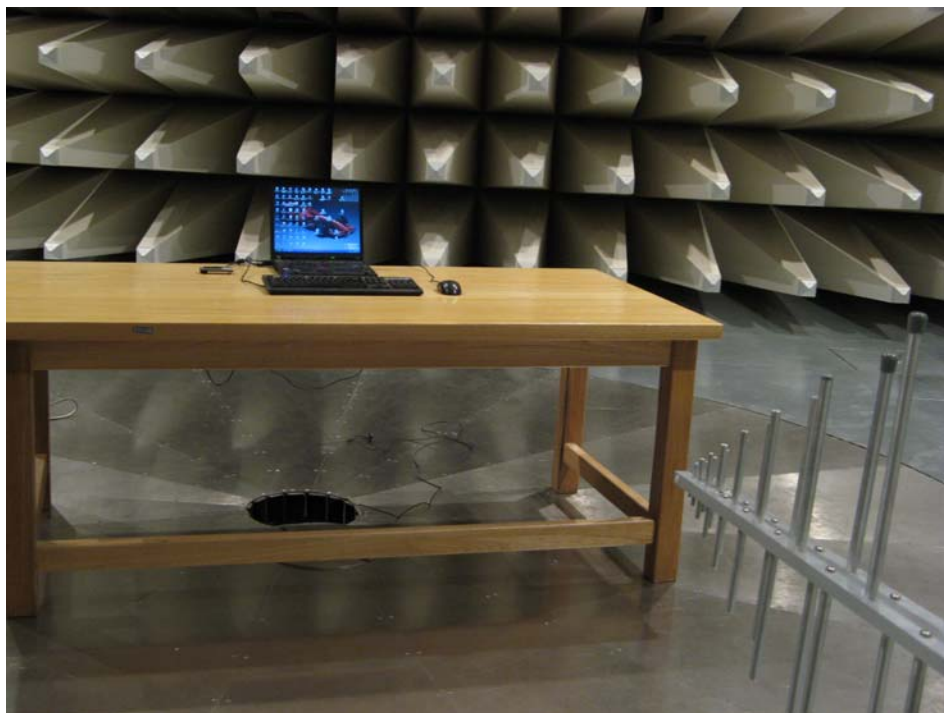
Pic 2 Radiated Spurious Emission Part15B
