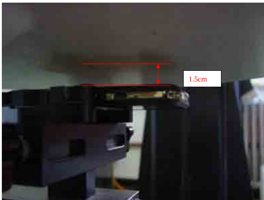
Picture B9: Body-worn Position (towards ground, the distance from handset to the bottom of the Phantom is 1.5cm)
