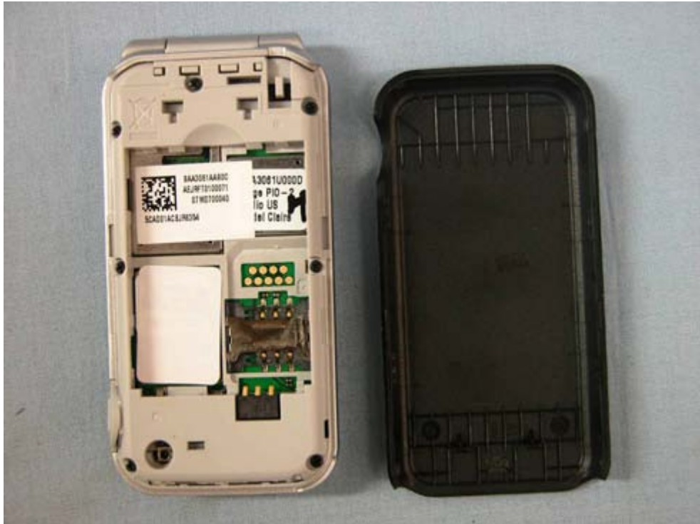
Mobile phone Disassembly
