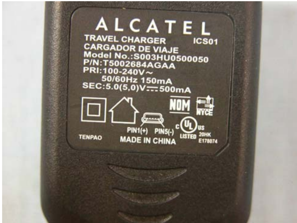
Label of Charger (AC/DC Adapter)
