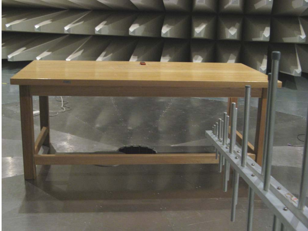
Pic 5 Part 15C Radiated Spurious Emission
