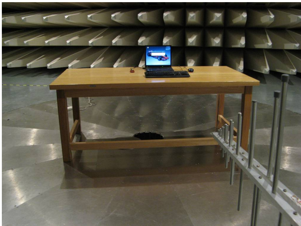
Pic 4 Part 15B Radiated Spurious Emission
