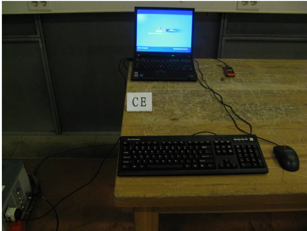
Pic 3 Part 15B Conducted Emission with laptop
