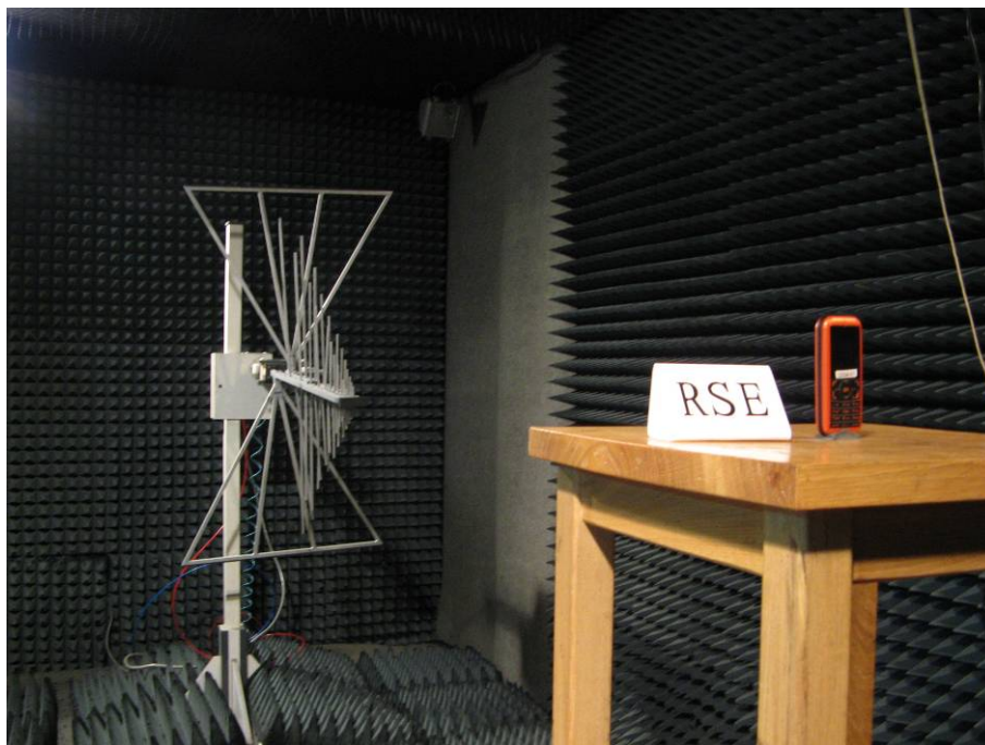
Pic 2 Part 2224 Radiated Spurious Emission
