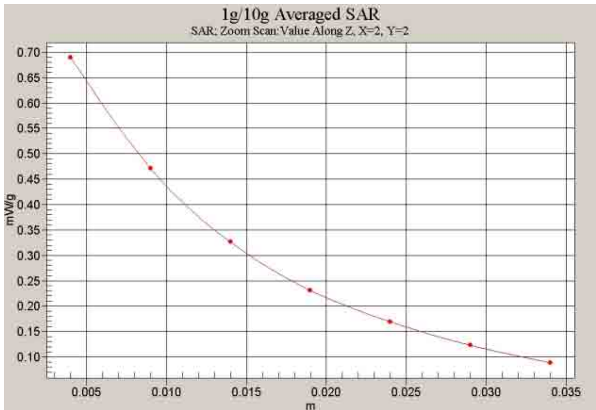
Fig. 16 Z-Scan at power reference point (850 MHz CH190)
