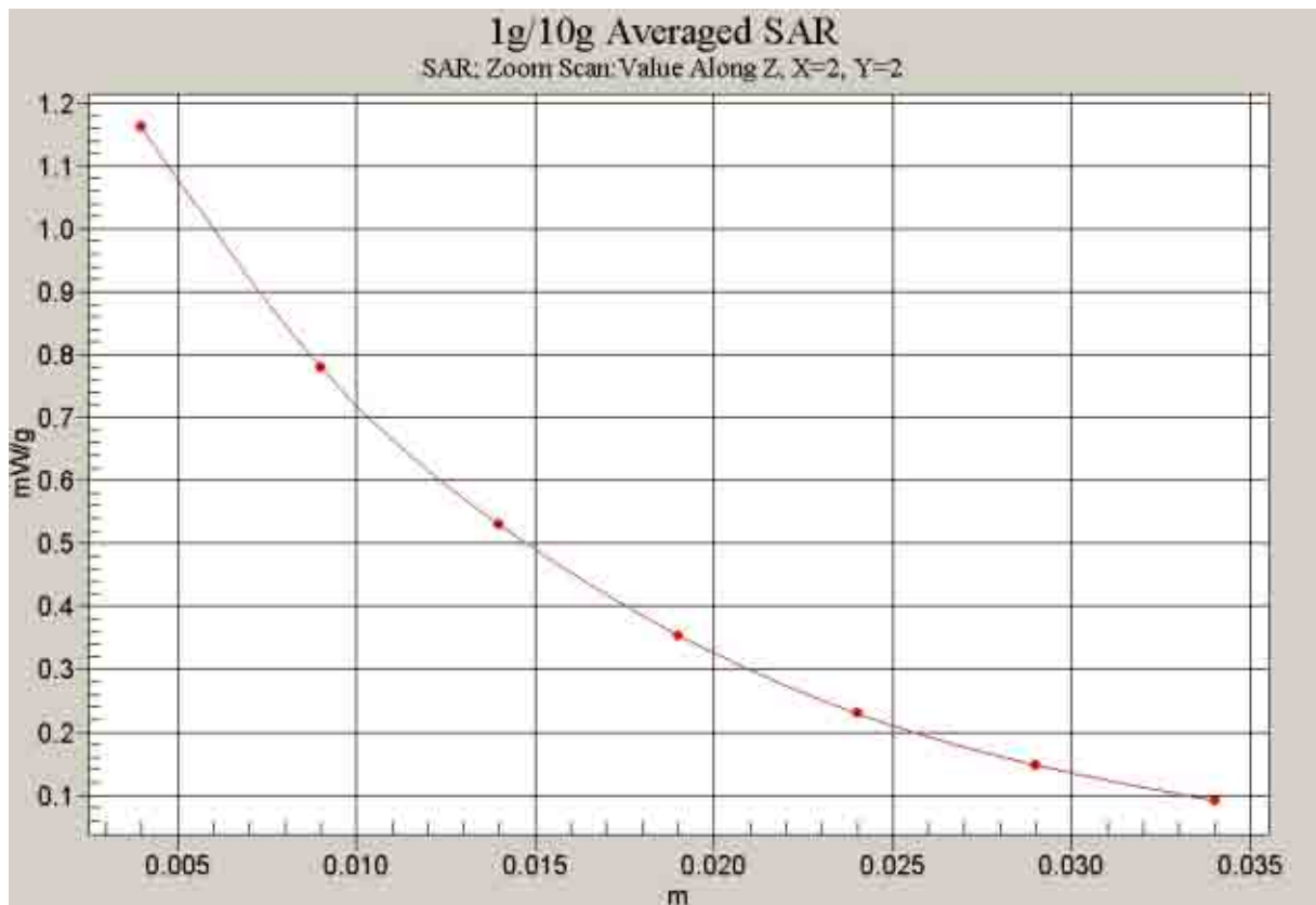
Fig. 34 Z-Scan at power reference point (1900 MHz CH661)
