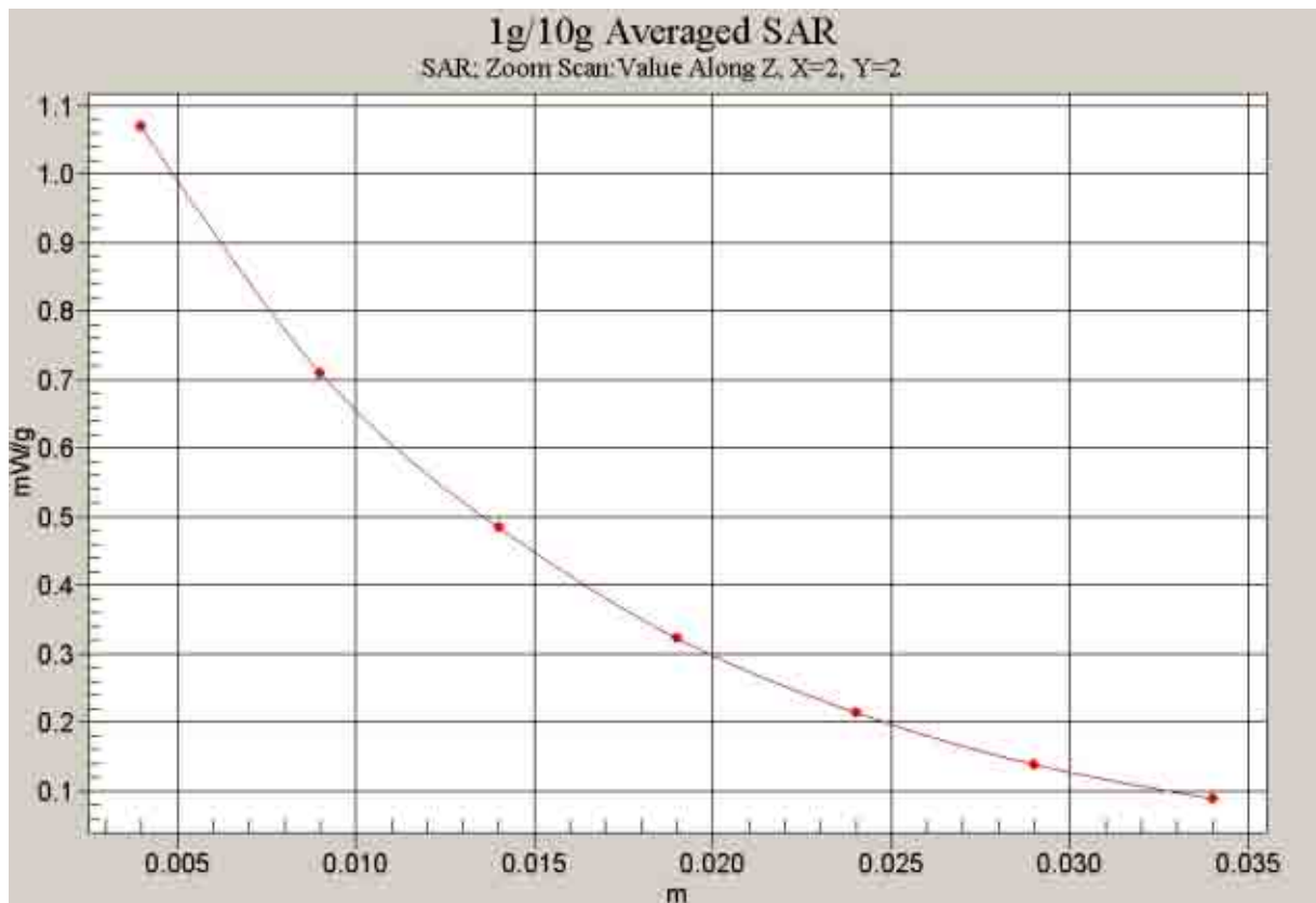
Fig. 32 Z-Scan at power reference point (1900 MHz CH810)
