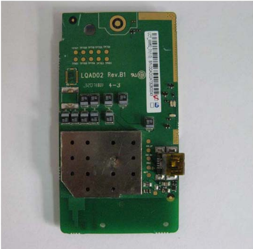
Picture 3: the top view of the sample with the RF shield-1
