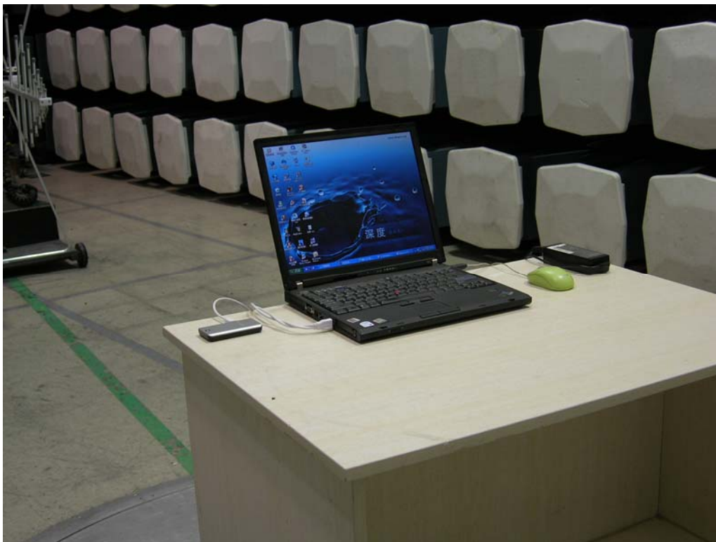
Figure RE for 15.109: Test Setup: 30MHz – 1GHz
