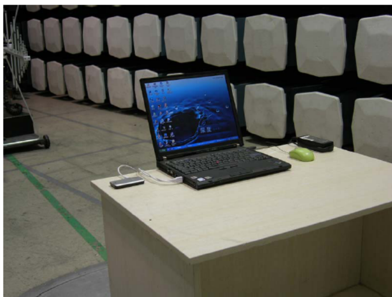
Figure RE for 15.109; Test Setup: 30MHz – 1GHz
