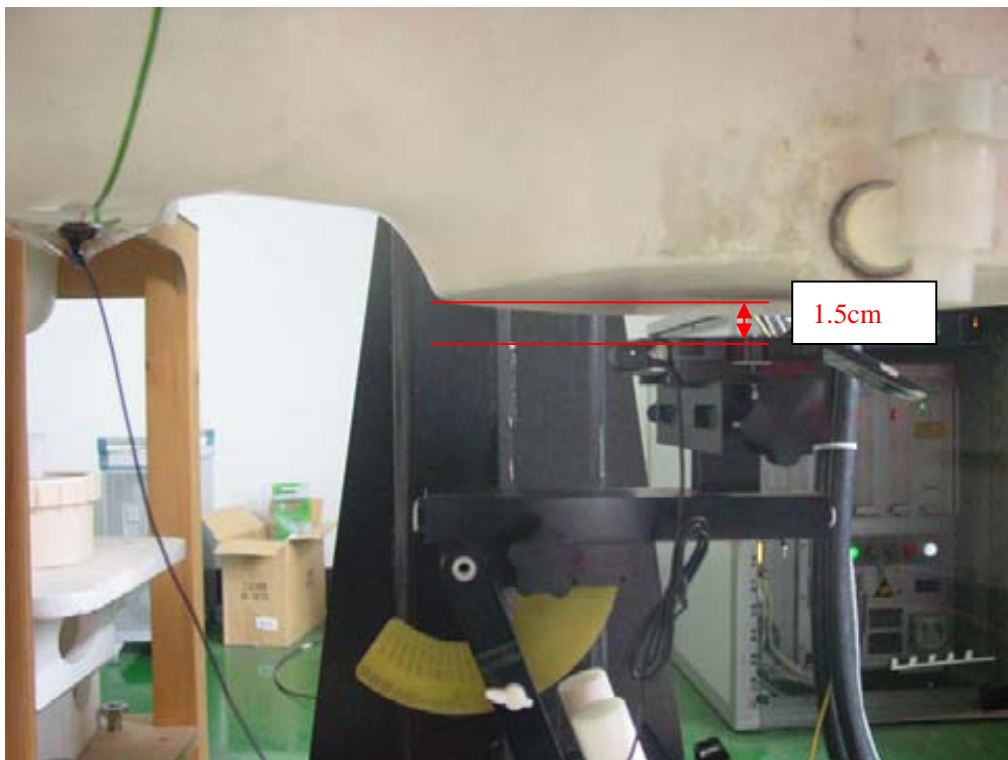
Picture B9: Body-worn Position (towards ground with headset, the distance from handset to the bottom of the Phantom is 1.5cm)
