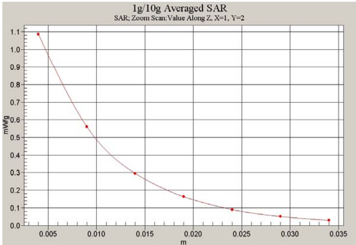
Fig. 44 Z-Scan at power reference point (1900 MHz CH512)
