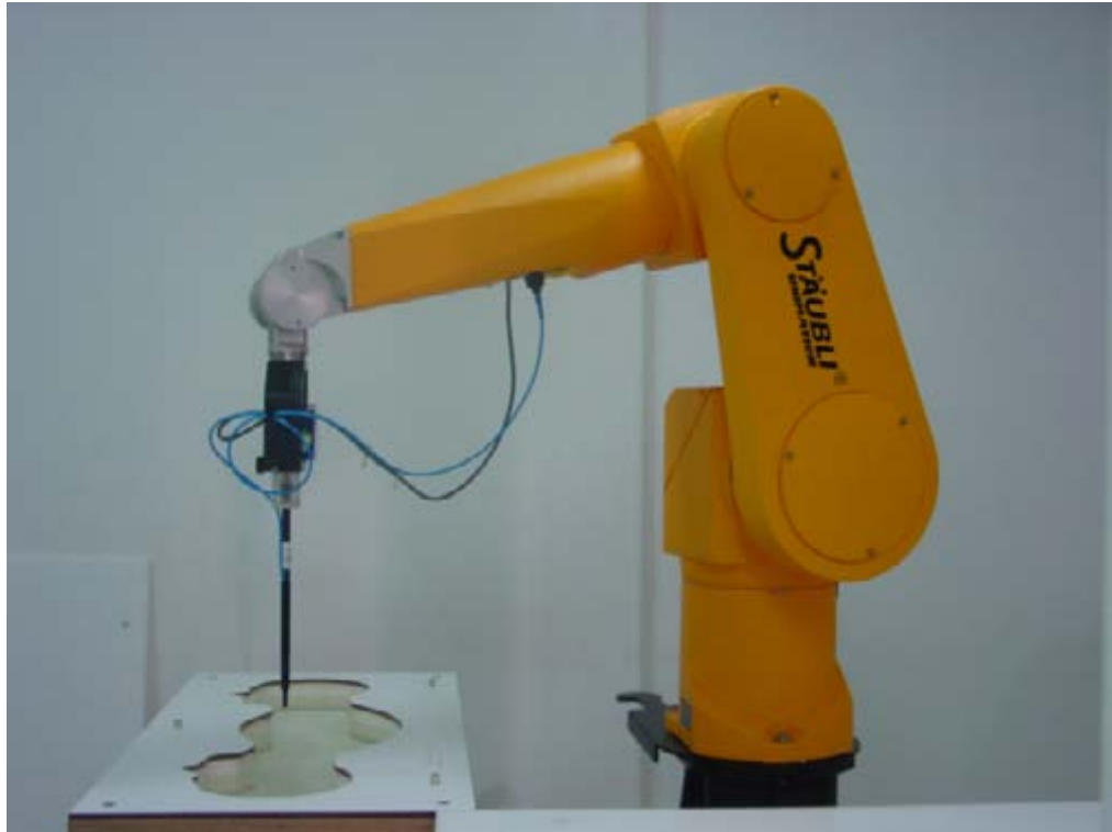
Picture B1: Specific Absorption Rate Test Layout
