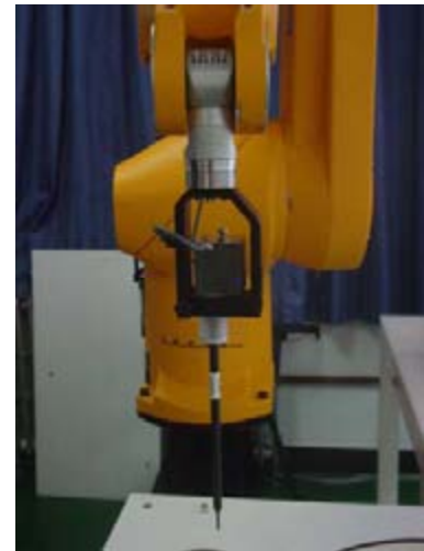
Picture4:ES3DV3 E-field probe
