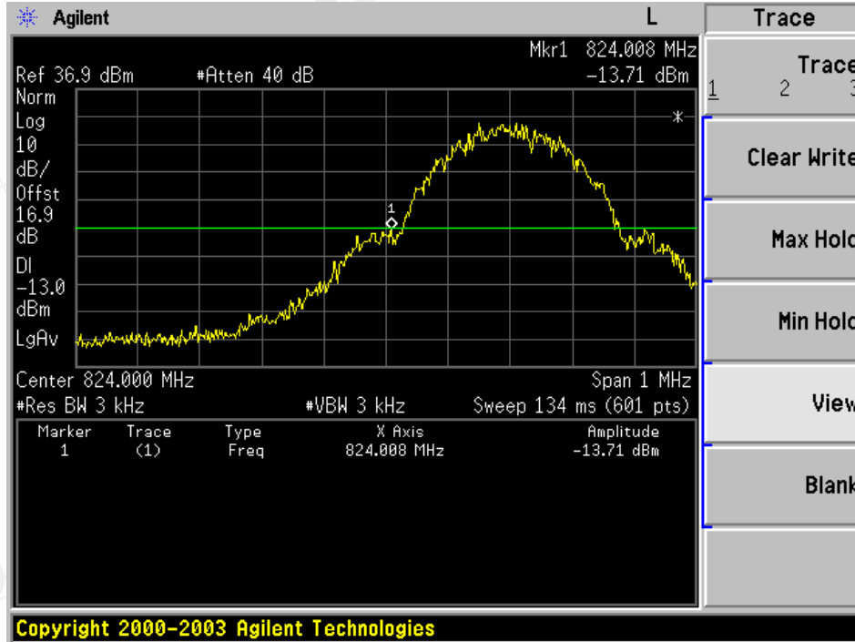
Figure 8-5: Band edge emission at antenna terminals – GSM Channel Highest
