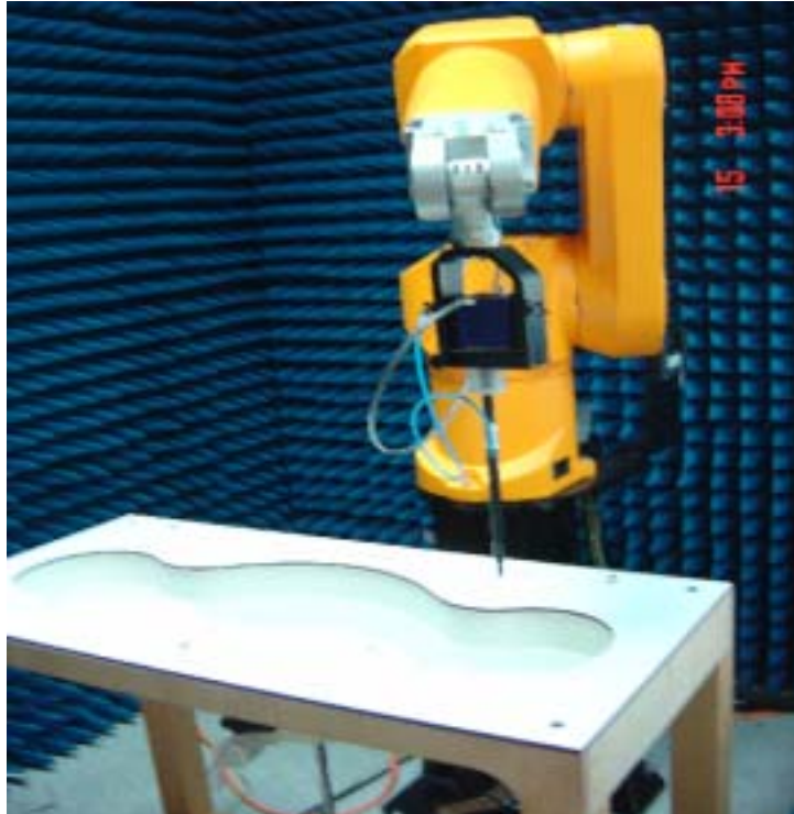
Fig.1 Photograph of the SAR measurement System
