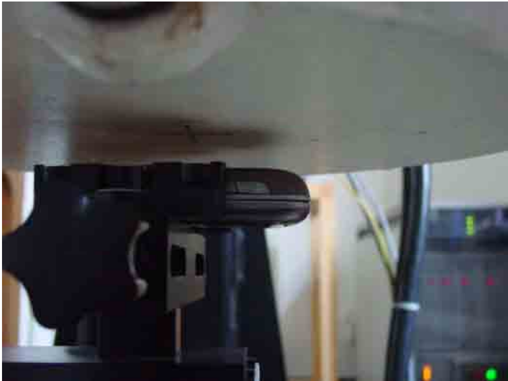
Picture B14: Body-worn Position with Slide down (towards ground, the distance from handset to the bottom of the Phantom is 1.5cm)
