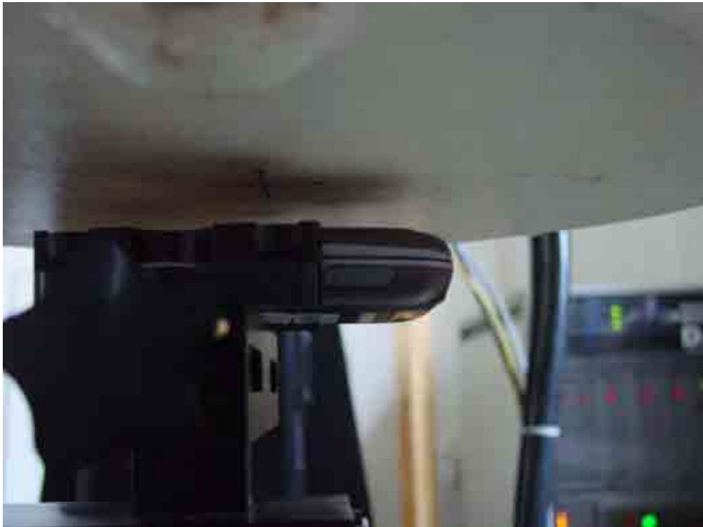
Picture B12: Body-worn Position with Slide down (towards phantom, the distance from handset to the bottom of the Phantom is 1.5cm)
