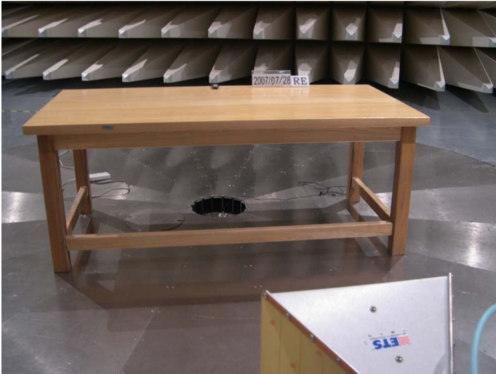
Photo of Radiated Emission Test
