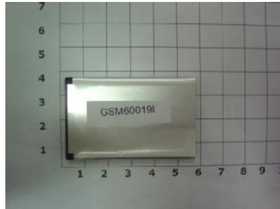
Fig.14 Back view of battery
