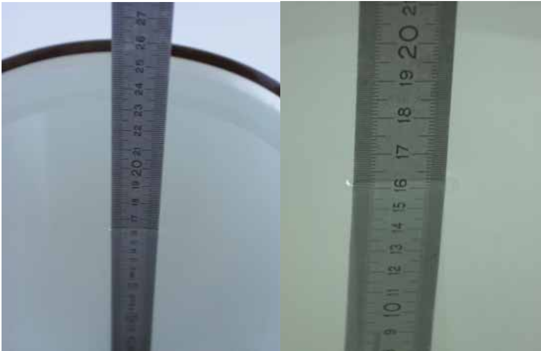
Fig. 22: Liquid depth for PCS 1900 Head and Body measurements.
