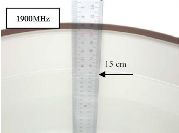
Fig.5 Photograph of the Tissue Simulant Liquid depth 15cm for Body-Worn
