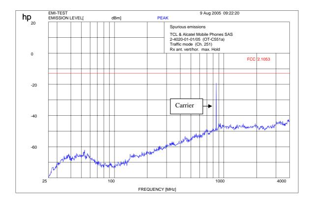
$\label{eq:generalized_states} \begin{array}{l} f < 1 \ GHz: RBW/VBW: 100 \ kHz \\ Carrier \ suppressed \ with \ a \ rejection \ filter \end{array}$
