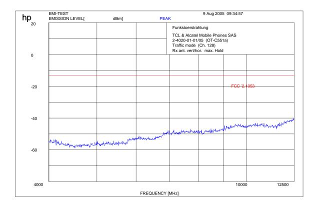
$\label{eq:generalized_formula} \begin{array}{ll} f < 1 \mbox{ GHz}: \mbox{RBW/VBW}: 100 \mbox{ kHz} & f \geq \\ \mbox{Carrier suppressed with a rejection filter} \end{array}$
