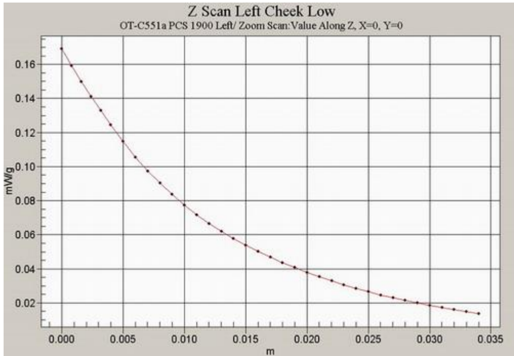
Fig. 26 Z-Scan at power reference point (Left Hand Touch Cheek 1900MHz CH512)
