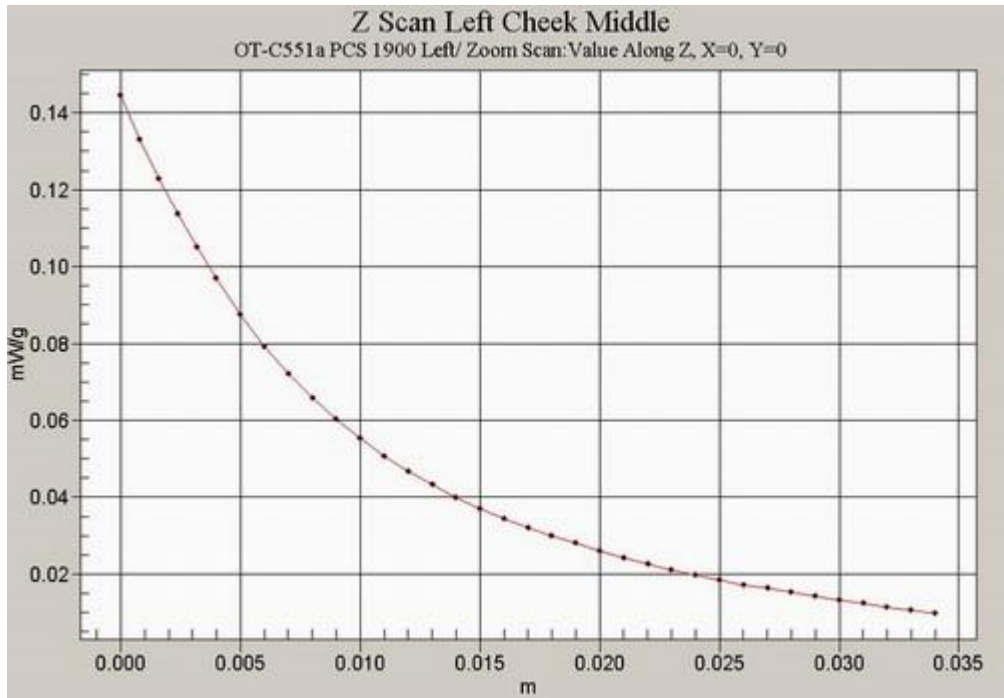
Fig. 28 Z-Scan at power reference point (Left Hand Touch Cheek 1900MHz CH661)
