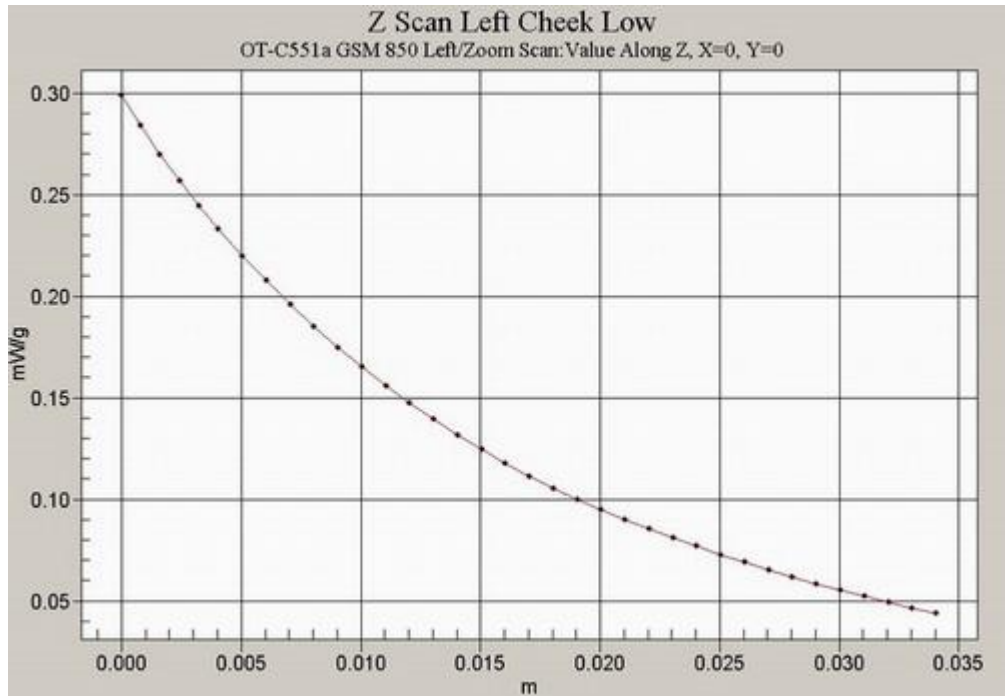
Fig. 2 Z-Scan at power reference point (Left Hand Touch Cheek 850MHz CH128)
