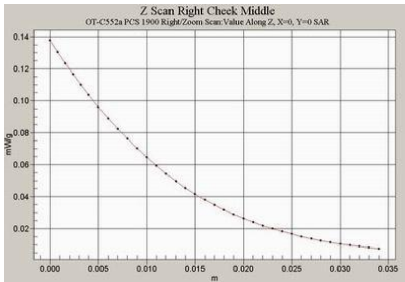
Fig. 40 Z-Scan at power reference point (Right Hand Touch Cheek 1900MHz CH661)
