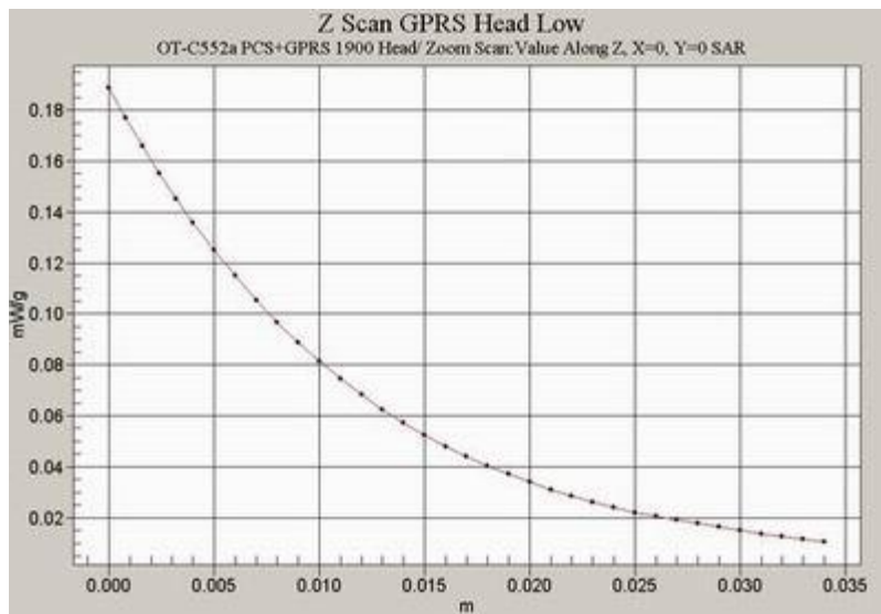
Fig. 104 Z-Scan at power reference point (Flat Phantom 1900MHz GPRS CH512 with the display of the handset toward the phantom)
