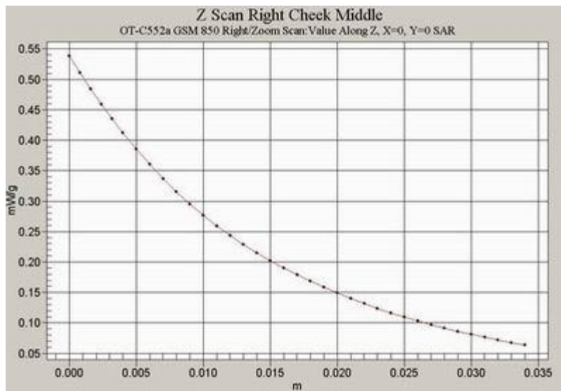
Fig. 16 Z-Scan at power reference point (Right Hand Touch Cheek 850MHz CH190)
