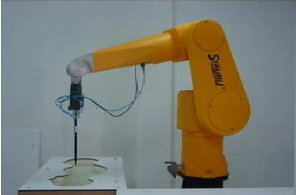
Picture 1 Specific Absorption Rate Test Layout
