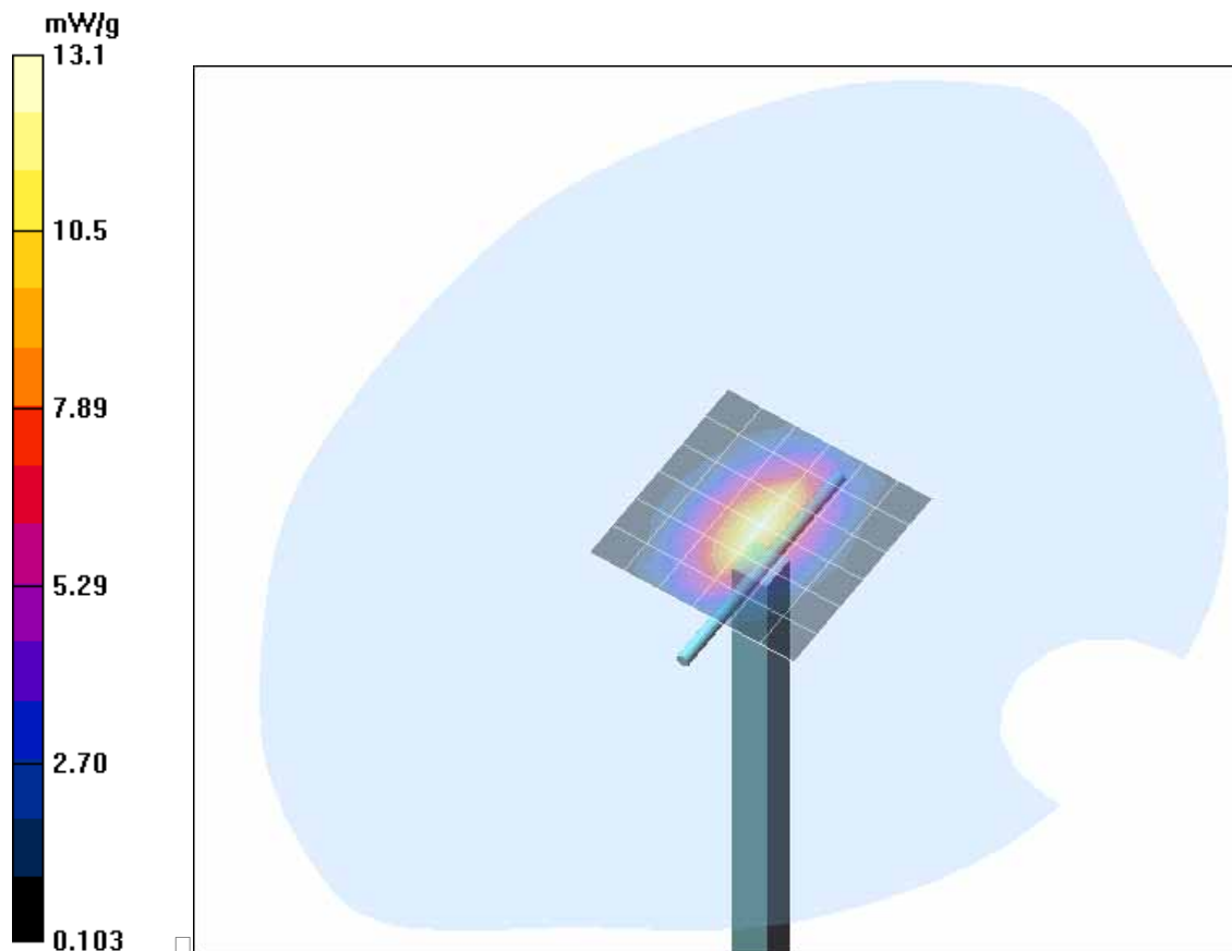
Fig. 15: Validation measurement 1900 MHz Body (July 07, 2005), coarse grid. Ambient Temperature: 22.0° C, Liquid Temperature: 21.0° C.
