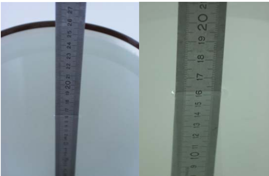
Fig. 23: Liquid depth for PCS 1900 Head and Body measurements.
