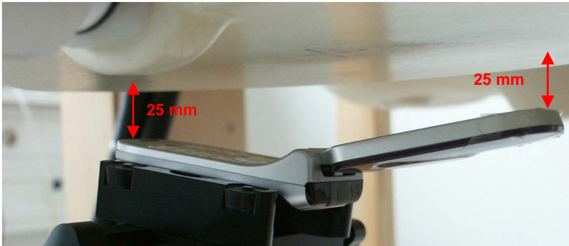
Fig. 22: Body worn configuration Alcatel OT-C651, PoC mode (GSM), display towards the phantom.
