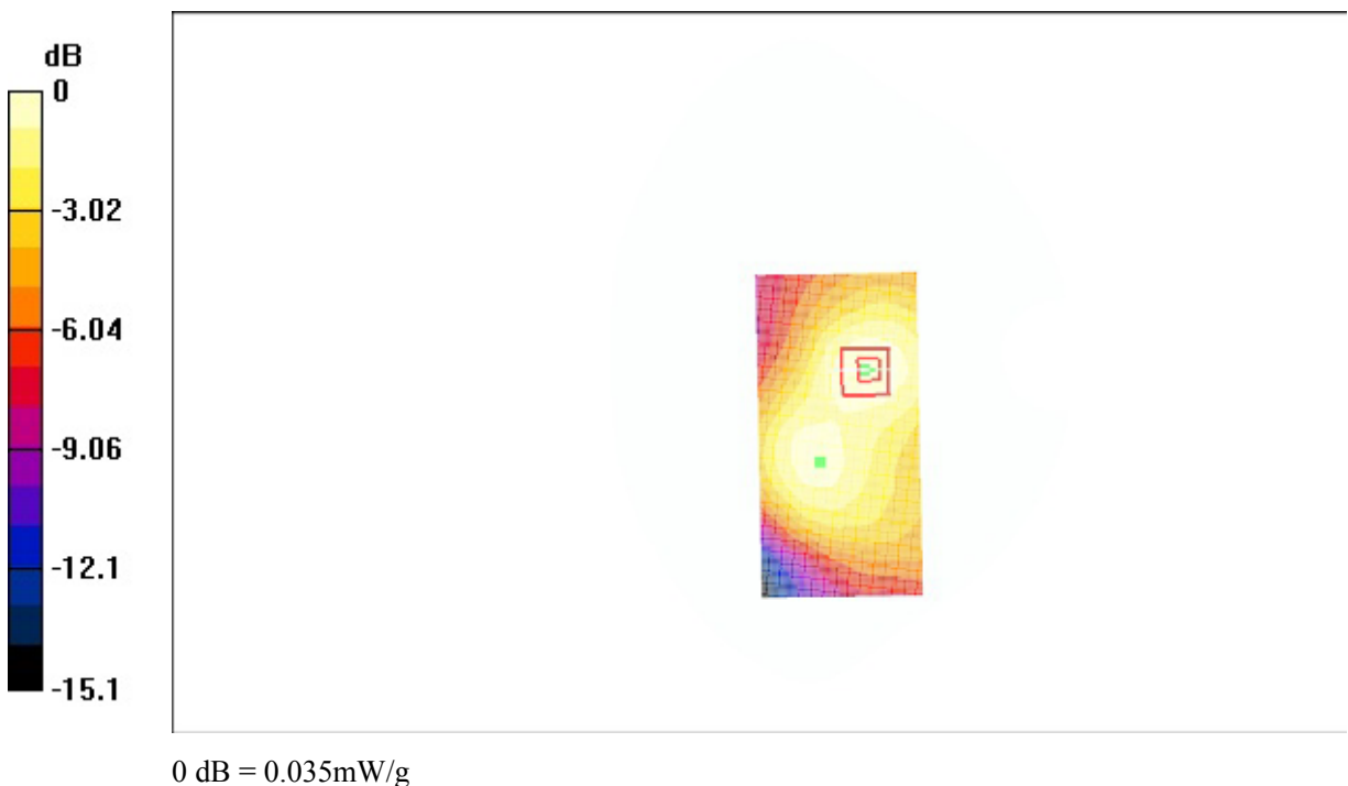
Fig. 25 Flat Phantom Body-worn Position 1900MHz earphone CH512 with the display of the handset towards the phantom
