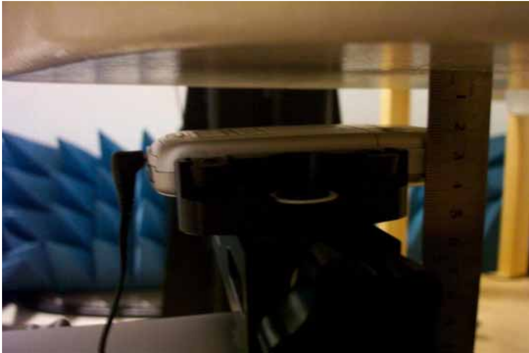
Picture 9 Flat Phantom -- Body-worn Position with earphone (toward ground, the distance from handset to the bottom of the Phantom is 2.0cm)
