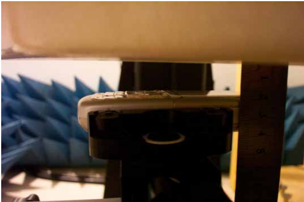
Picture 10 Flat Phantom -- Hand-worn Position (toward phantom, the distance from handset to the bottom of the Phantom is 2.0cm)
