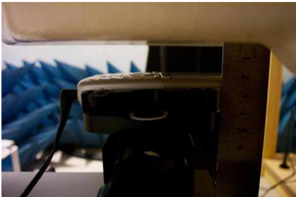
Picture 8 Flat Phantom -- Body-worn Position with earphone (toward phantom, the distance from handset to the bottom of the Phantom is 2.0cm)
