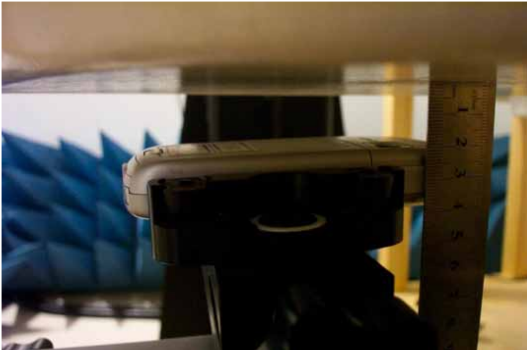
Picture 7 Flat Phantom -- Body-worn Position (toward ground, the distance from handset to the bottom of the Phantom is 2.0cm)
