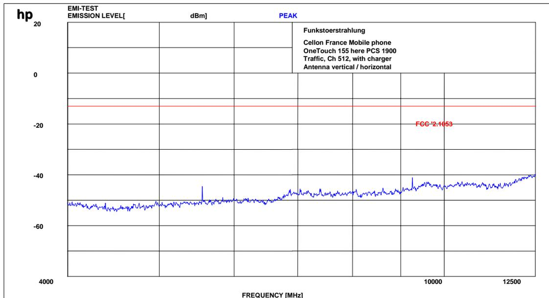
The measurements were performed up to 20 GHz with a special low-noise preamp and a wideband horn antenna. There were no spurs found.
