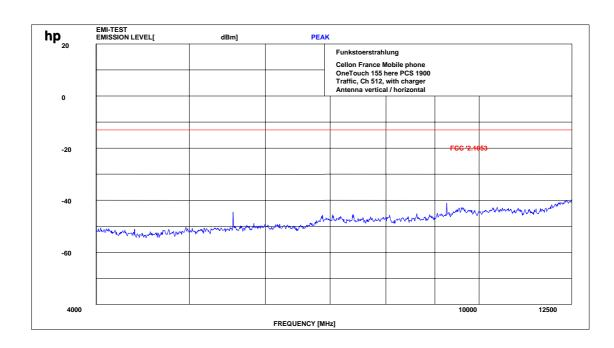
The measurements were performed up to 20 GHz with a special low-noise preamp and a wideband horn antenna. There were no spurs found.
