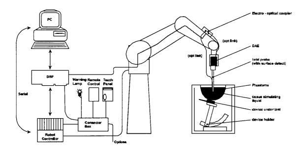
The DASY4 system for performing compliance tests consists of the following items:
