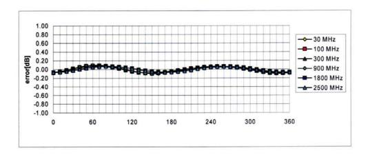
Axial Isotropy Error < ± 0.2 dB
