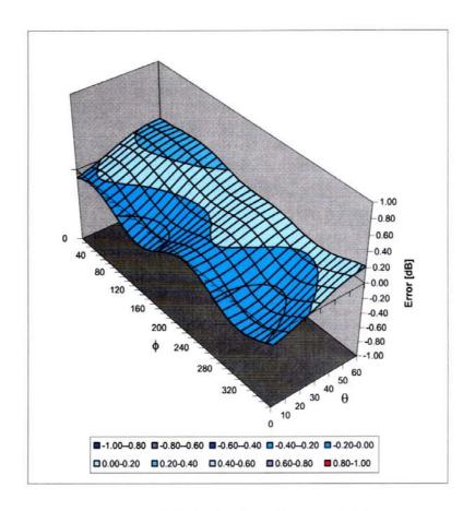
Spherical Isotropy Error < ± 0.4 dB
