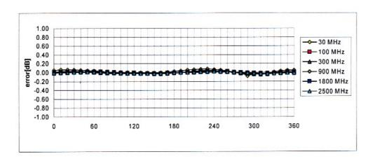
Axial Isotropy Error < ± 0.2 dB
