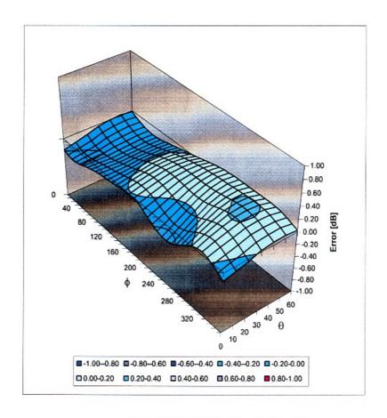
Spherical Isotropy Error < ± 0.4 dB
