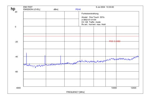
$f < 1 \ GHz : RBW/VBW: 100 \ kHz$   $f \ge 1GHz : RBW/VBW: 1 \ MHz$  Carrier suppressed with a rejection filter
