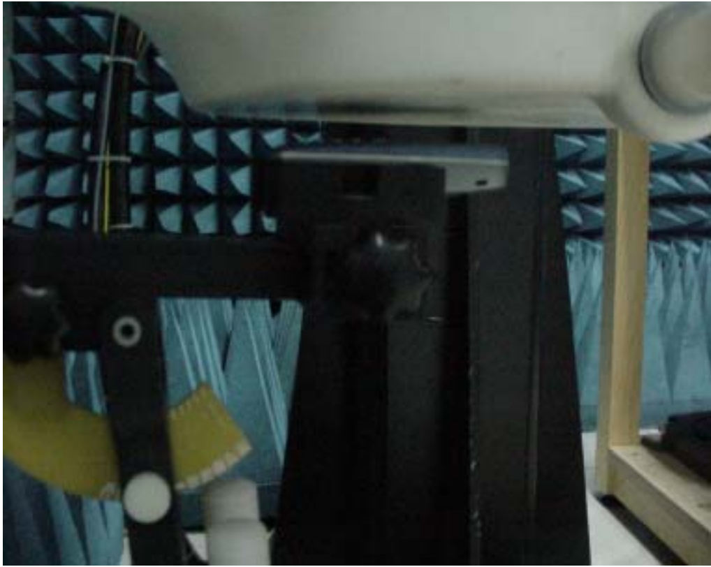
Picture 6 Flat Phantom -- Body-worn Position (toward phantom, the distance from handset to the bottom of the Phantom is 1.5cm)
