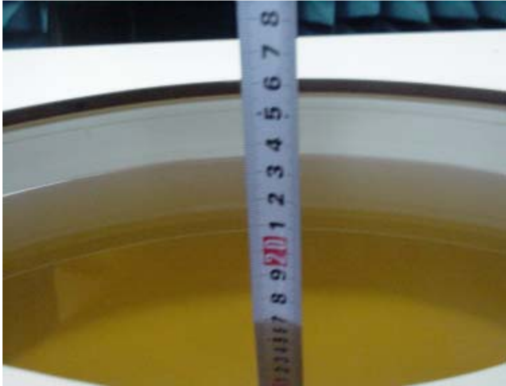
Picture 9 Liquid depth in the Flat Phantom (Body 850MHz)
