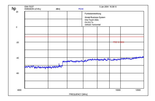
f < 1 GHz : RBW/VBW: 100 kHz f? 1GHz : RBW / VBW 1 MHz
