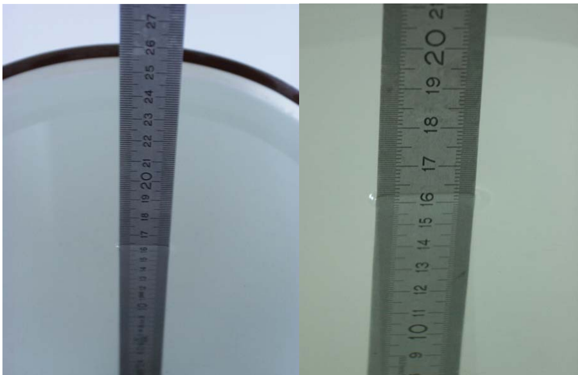
Fig. 32: Liquid depth for PCS 1900 Head and Body measurements.
