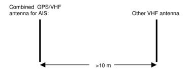
Vertical separation distance and distance from mast or other object of metal:
