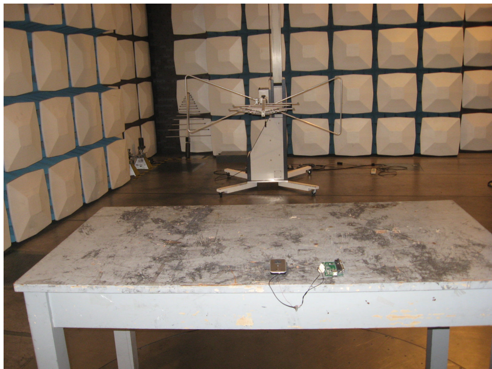
Photograph 2: Set-up for Spurious Emissions (30MHz-1GHz)
