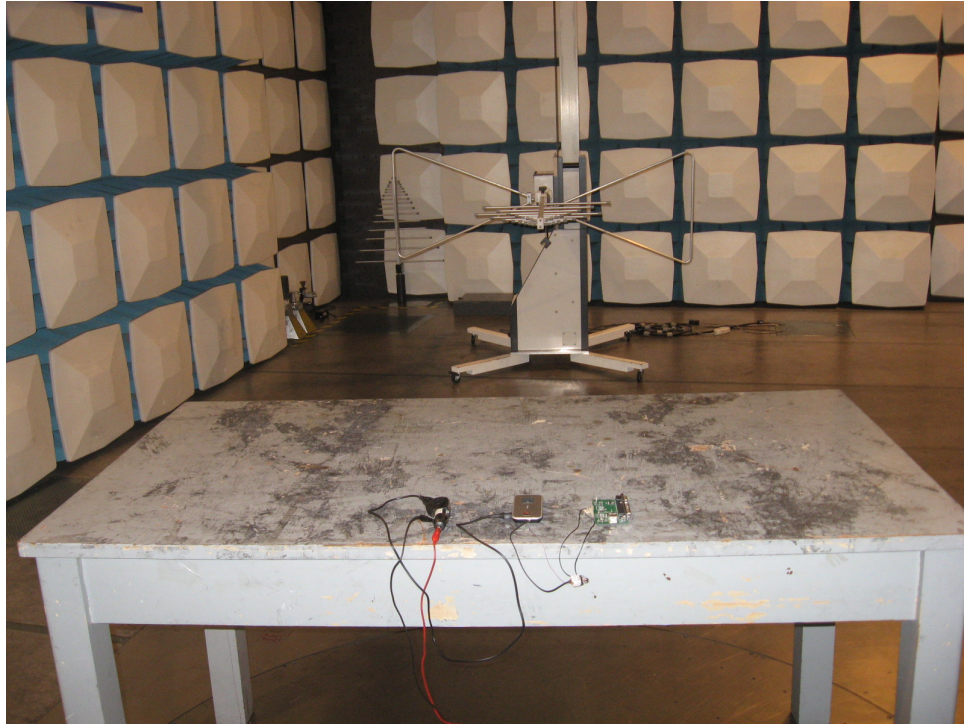
Photograph 5: Set-up for Radiated Emissions
