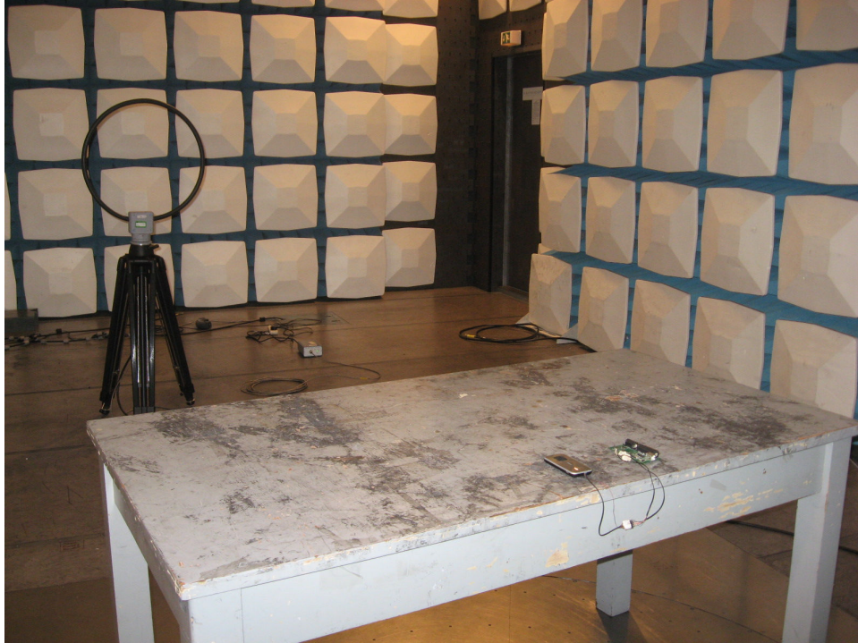
Photograph 2: Set-up for Spurious Emissions (30MHz-1GHz)
