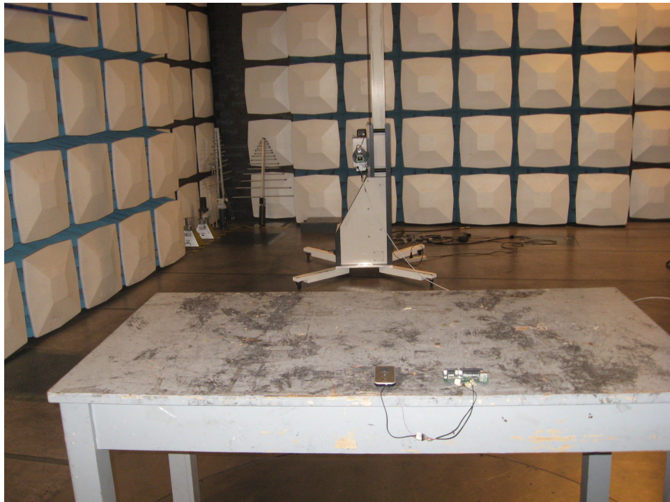
Photograph 4: Set-up for Spurious Emissions (18GHz-26GHz)
