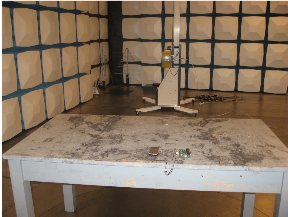
Photograph 4: Set-up for Spurious Emissions (18GHz-26GHz)
