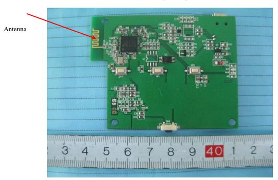
**EUT – Main Board Top Components View**
