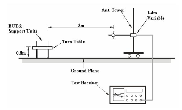
The radiated emission tests were performed in the 3 meters chamber B test site, using the setup accordance with the ANSI C63.4-2003. The specification used was the FCC 15.205; 15.209 and FCC 15.247 limits.
