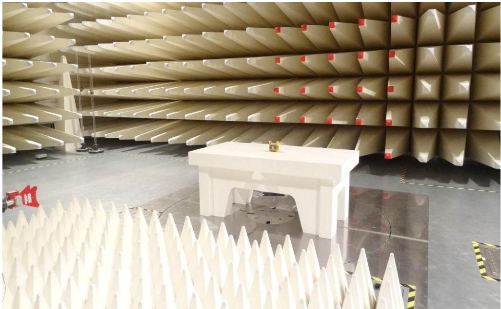
Radiated Test setup
