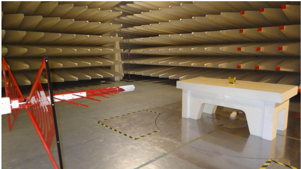
Radiated Test setup
