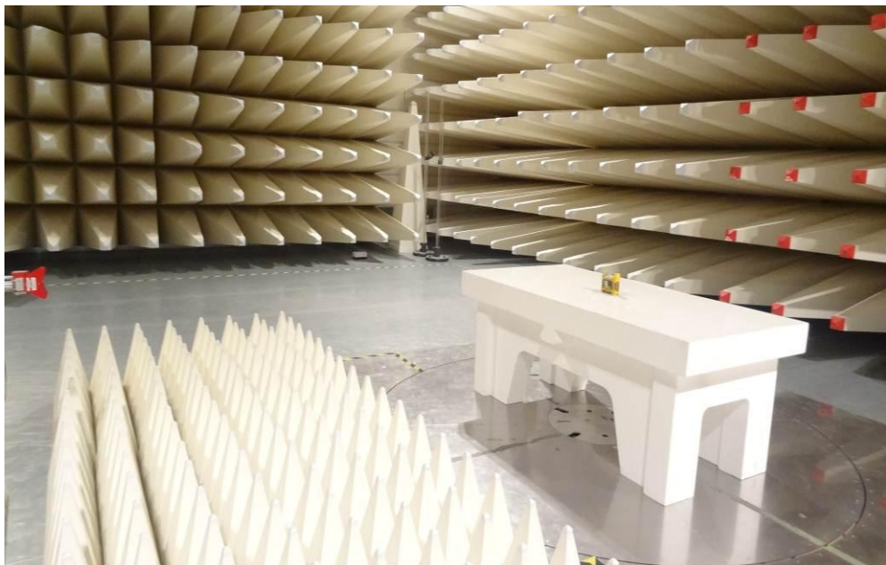
Radiated Test setup
