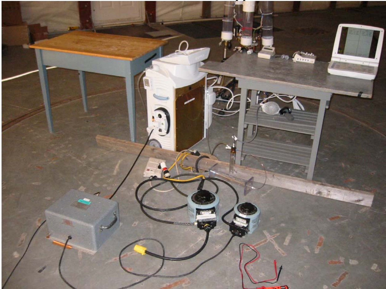
Line-Conducted Emissions, Front View, Ventricular Assist Mode
