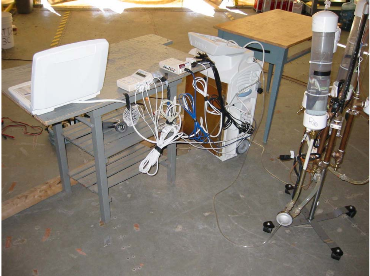
Line-Conducted Emissions, Back View, Balloon Pump Mode
