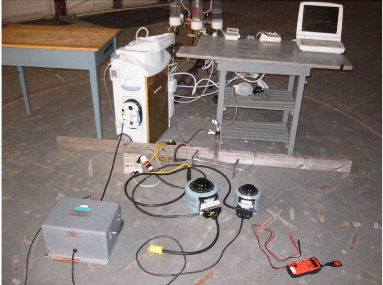
Line-Conducted Emissions, Front View, Balloon Pump Mode
